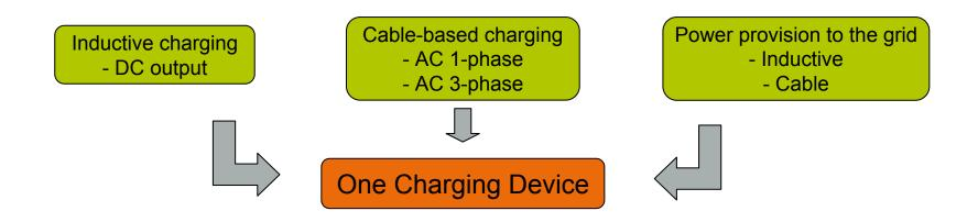
Actual functionality of the laboratory prototype (Fraunhofer IWES):
